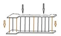
4. Use BOUNCING BOARD and hammer to hit parts together.
