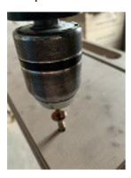
6. Make marks on the wall – copy them froms left side (inside), copy them from right side (outside): those will be the centers for drill holes, drill (with 12mm drill) holes 60mm deep, hit in plastic dowel, use screw A4 with electric screw driver, in the finish use wrench 13mm to screw the nut.
